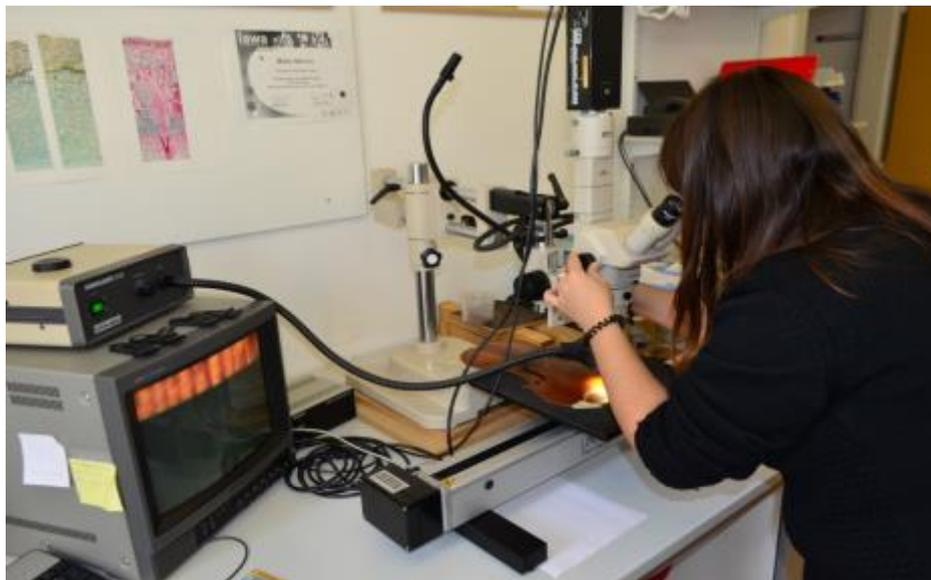
Fig.6. Measuring tree-ring width on the violin belly with LINTAB measuring table and TSAP Win software
