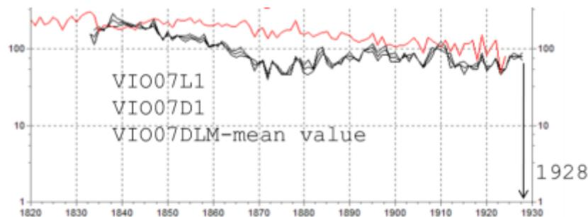
Fig.7. Tree-ring series of the violin (black) with the last ring dated to 1928, the reference chronology (red) and the end year 1928.
