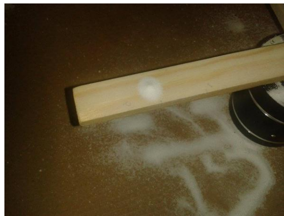
Picture 2. Chladni pattern on vibrating sample (combined flexural vibration, about both minor and major axis, and torsional vibration)
