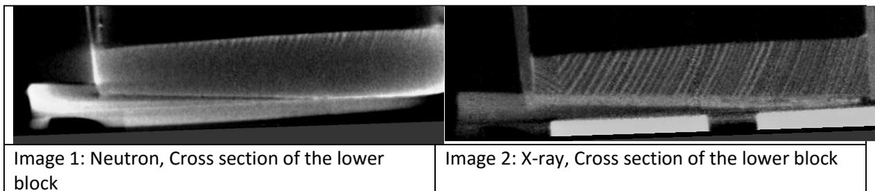
In the X-ray cross sections of the lower block and the neck joint, one can see that the block is made out of two pieces with different orientation of the annual rings and the top plate is fixed by a nail in the upper part. A cross section of the neutron image through the ribs does not show the bevelled joint of the ribs in the corners. This technical detail is visible in the X-ray image.
